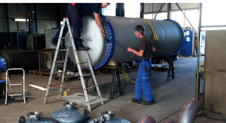
Lorch SpeedRoot: Spatter-free and with very low energy input, SpeedRoot closes even eight-millimetre gaps in root welding three times faster than TIG processes.
