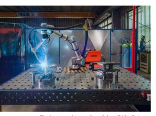
The large working radius of the UR10e Cobot from the Lorch Cobot Welding World and the Smart Copy programming function offer ideal prerequisites for smooth production sequences.
