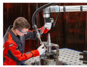
The innovative multifunctional flange and three freely assignable buttons permit direct integration of the practical additional Quick-Points feature for speedy teaching of parts on the Cobot.
