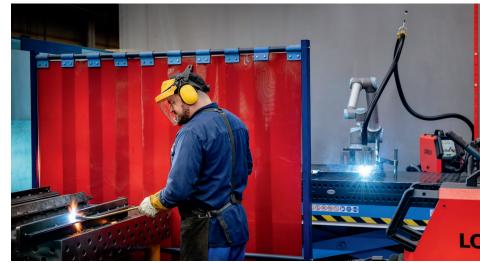
Time savings: The welder is already preparing the next part for welding while the Lorch Cobot accurately applies the weld seams set for recurring parts.
