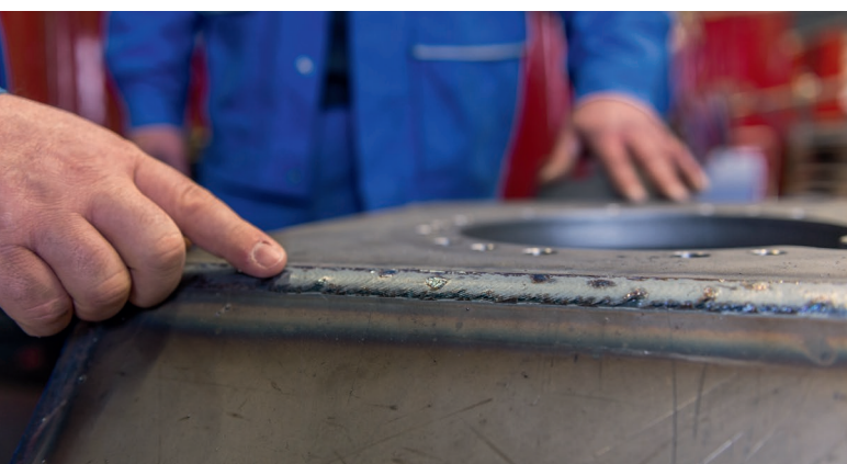
Best surfaces, virtually spatter-free: Robots have reduced the amount of rework per weld seam to an absolute minimum.
