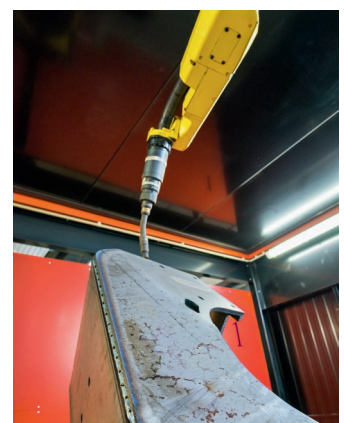
Smart: The robot always finds the ideal weld path with the help of the seam tracking function.
