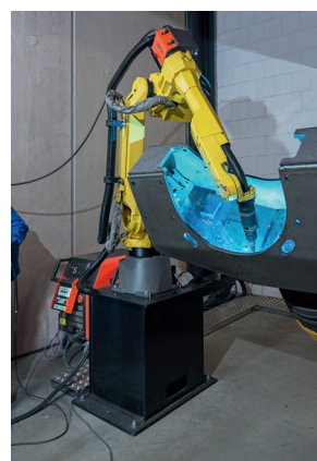
Flexible: Welding is always possible in the optimal position of the tray due to the precise interaction of the robot arm and positioner.
