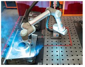
Optimal structure: The cobot in between two standard workstations. Three set-ups are enough to weld any weld seams of the turbine housing easily this way.
