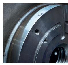
Perfect circumferential weld seam: The ring can be welded to the turbine chassis in a quality never seen before with the Cobot in spite of the difficult chassis (manganese steel).
