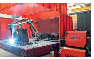
The entire welding machinery, including the Lorch welding Cobot that is mainly used to efficiently weld turbines made of manganese steel, is connected to Lorch Connect.
