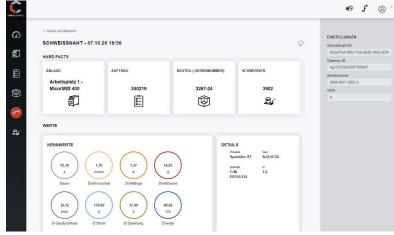
Every individual weld seam is documented with the associated parameter values. Any anomalies or deviations can be corrected quickly this way. The dashboard quickly and clearly displays all important production key figures, such as arc times, wire consumption, or energy consumption. This allows Rösler to always keep an eye on productivity.
