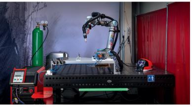
Highest possible safety during series production: An installed scanner safety system with audible and visual warning signals and an emergency stop function protect the operator from potential hazards while welding.
