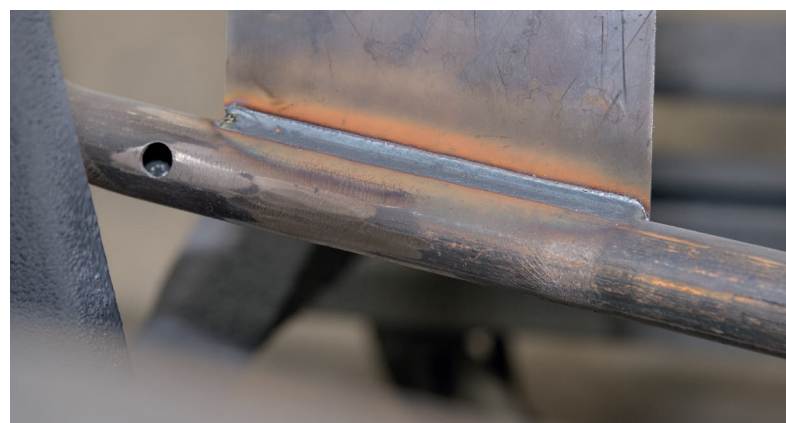
Thin steel plates with thicknesses between 1.0 and 1.6 millimetres are welded to the base frame. The Lorch SpeedCold welding process only applies the energy currently required.
