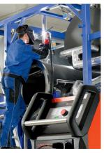
An end to unnecessary walking: Digital data coupling allows control of the most important welding parameters from the torch, even while the system is not in view. The figure shows the T300 AC/DC, which is optimised for industrial TIG production.
