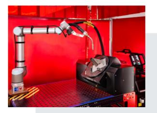
"Thanks to the welding cobot solution with tilt-turn table, we have been able to achieve massive time savings of up to 40% in series parts. We also relieve our welders in particular of long, exhausting welding work."
