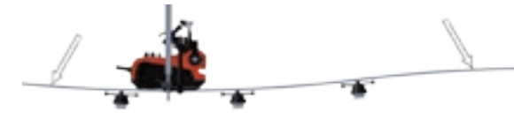
Welding on a concave plane with Flex guide rail
