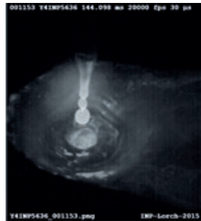
The primary droplet enters the weld pool, and the secondary droplets detach.
