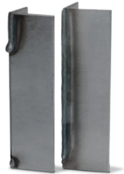
A welded corner seam as a comparison. Standard arc (left): Rapidly falling weld pool that is about to drop off. SpeedCold (right): Welded in full with utmost speed and reliability (35 cm/min).
