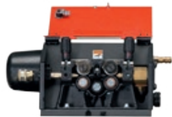
4-roll precision wire feeder with robust, weight-optimised feed plate made of plastic reinforced with fibreglass and with a change of rolls without tools.
