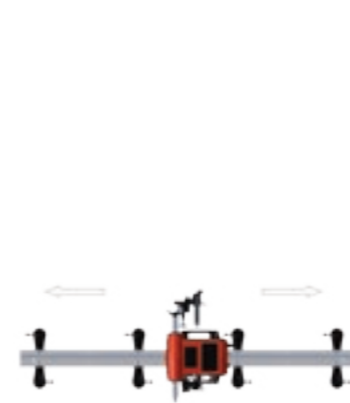
Welding in the horizontal position with guide rails (laterally with magnetic holders)
