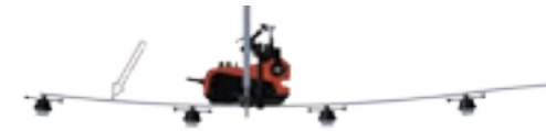
Welding on a concave plane with Flex guide rail (tank \varnothing 10 m or greater)
