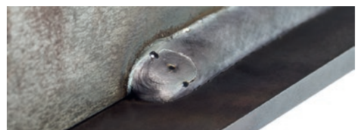
With crater filling – perfect end of weld seam.
