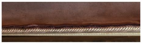
MicorTwin stainless steel fillet weld 6 mm
